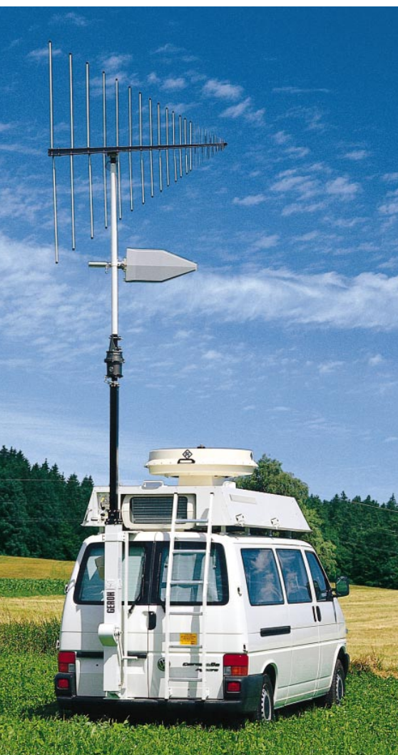
FIG 1 DF and monitoring vehicle with VHF-UHF Direction Finder DDF190. With its upper frequency of 3 GHz, DDF190 can also detect sources of interference affecting new radio services (eg GSM, PCN, PCS, WLL and GPS).
