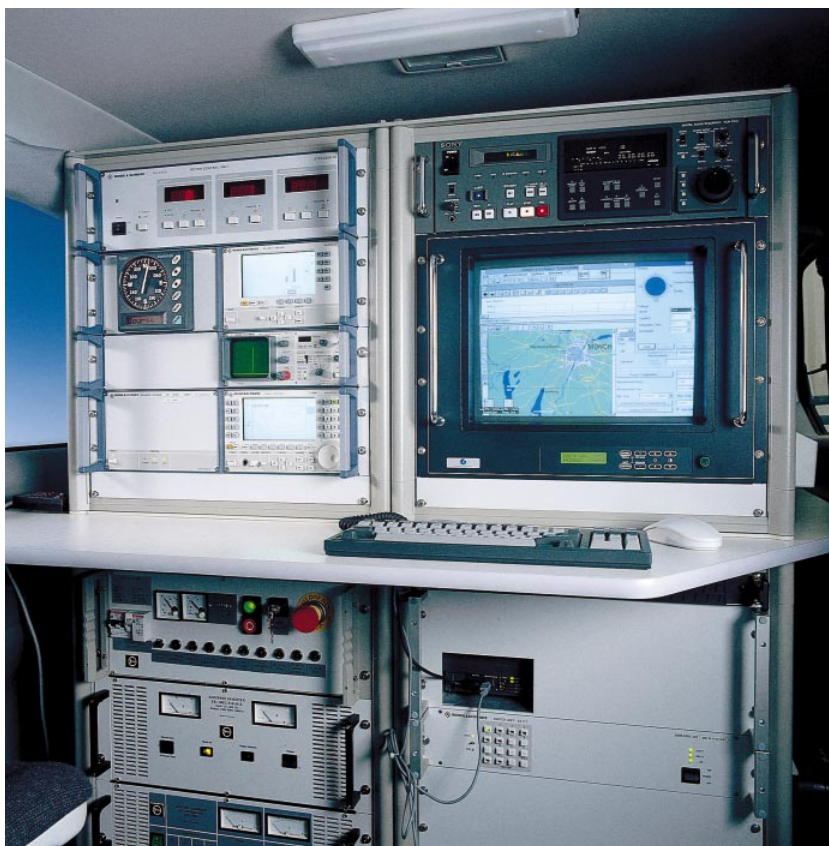
FIG 2 DDF190 upgrades VHF-UHF receivers to top-end DF system – with accuracy and sensitivity above 1 GHz unrivalled by any other compact unit. Photo 42 571/1
