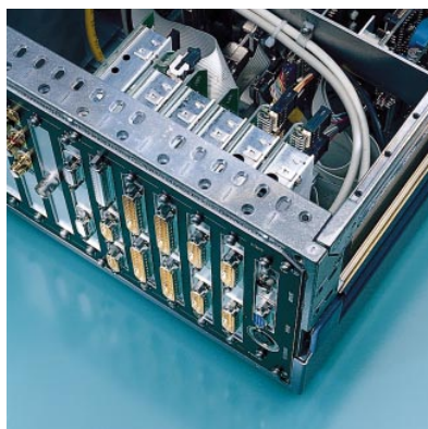
FIG 2 EMC filters in serial and parallel interfaces of System Processor MERLIN GR2000X
