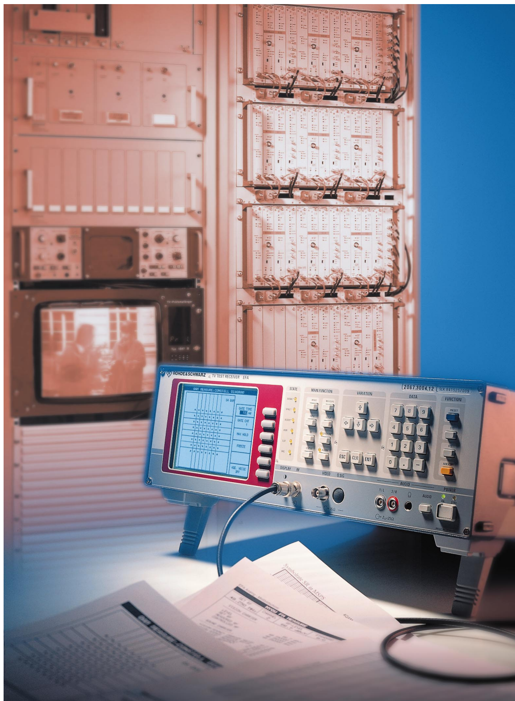
FIG 1 TV Test Receiver EFA, allround specialist for measurements on analog and digital TV signals – seen here in headend station Photo 42 575
